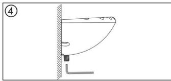
① Ensure soap dish is level. ② Fix support in place: ensure screws and rawl plugs are suitable for wall type. ③ Clip soap dish onto support. ④ Tighten grub screw using a 3mm Allen key.
