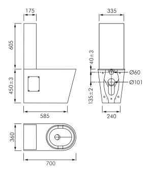
Supplied as standard P trap, it can be converted to S trap using a proprietary waste elbow.
