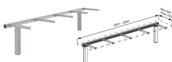
INDIVO lift for worktop, with two motors and control box. Incl. cross brace and five brackets. Height adjustable up to 300 mm with switch or wired remote control. For worktop length 2401-3000 mm.
