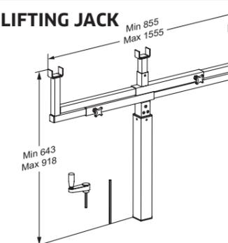
Crank-operated raiser for fitting with brackets for worktop RK1100/RK1101. Can adjust the height of the worktop with up to 250 mm.
