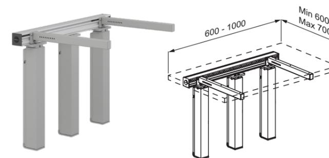
INDIVO lift for worktop, with three motors and control box. Incl. cross brace and two brackets. Height adjustable up to 300 mm with switch or wired remote control. For worktop length 600-1000 mm.
