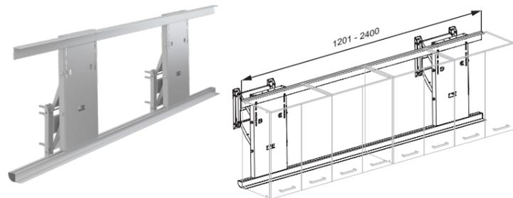
INDIVO lift for wall cupboards, with two motors and control box. Height adjustable 430 mm with switches or wired remote control. When height adjusting downward, the lift will also move 180 mm towards the user. For wall cupboards width 1201-2400 mm.
