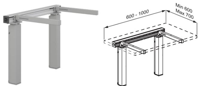
INDIVO lift for worktop, with two motors and control box. Incl. cross brace and two brackets. Height adjustable up to 300 mm with switch or wired remote control. For worktop length 600-1000 mm.
