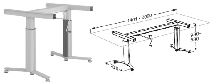
Manual lift for freestanding worktop. For worktops from 1400 - 2000 mm. Height adjustable 300 mm. Including 2 telescopic legs, longitudinal and cross braces and crank handle.
