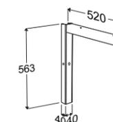
Bracket for worktop. Including 1 wall fitting and 1 carrying bracket. Height adjustable 250 mm.
