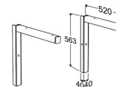
Bracket for worktop Including 2 wall fittings and 2 carrying brackets. Height adjustable 250 mm.
