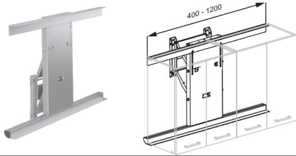
INDIVO lift for wall cupboards, with one motor and control box. Height adjustable 430 mm with switches or wired remote control. When height adjusting downward, the lift will also move 180 mm towards the user. For wall cupboards width 400-1200 mm.
