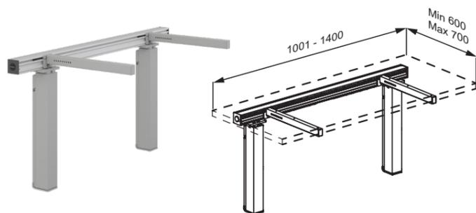
INDIVO lift for worktop, with two motors and control box. Incl. cross brace and two brackets. Height adjustable up to 300 mm with switch or wired remote control. For worktop length 1001-1400 mm.
