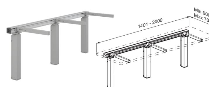
INDIVO lift for worktop, with three motors and control box. Incl. cross brace and three brackets. Height adjustable up to 300 mm with switch or wired remote control. For worktop length 1401-2000 mm.
