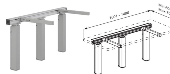
INDIVO lift for worktop, with three motors and control box. Incl. cross brace and two brackets. Height adjustable up to 300 mm with switch or wired remote control. For worktop length 1001-1400 mm.
