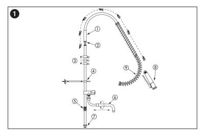
(1) Reinforced flexible hose, to attach to the column / (2) Anti-torsion, rotating nut / (3) Stainless steel spring guide for height adjustment / (4) Reinforced fixing bracket / (5) Information sticker: "Turn-off after use" / (6) Telescopic or S-shaped / (7) Rotating nut for fixing the column onto the valve / (8) Trigger-operated hand spray / (9) Spring (ensure that the spring direction is maintained).
