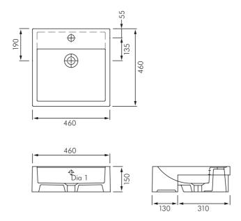
Semi recessed basin is designed to be fitted to suitably constructed bench that will allow for cutout required as per template supplied.
