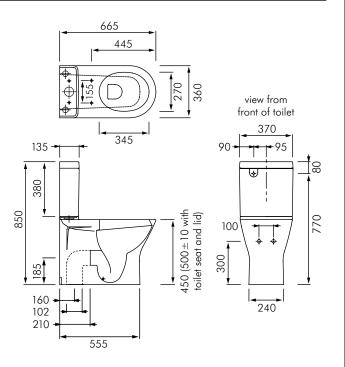
**Fixing:** FS37UK floor fixing kit included. **Cistern:** 4.5/3L dual flush, fitted directly to toilet pan with concealed fixings. Optional button set to prevent unwarranted lid removal.
