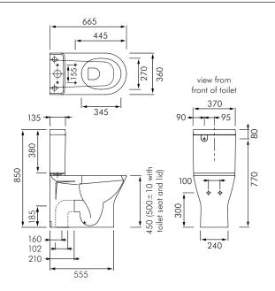
**Cistern**: 4.5/3L dual flush, fitted directly to toilet pan with concealed fixings. Optional button set to prevent unwarranted lid removal.
