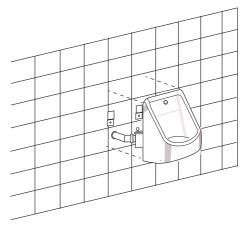
Fit threaded waste insert using tightening tool supplied (see right)
