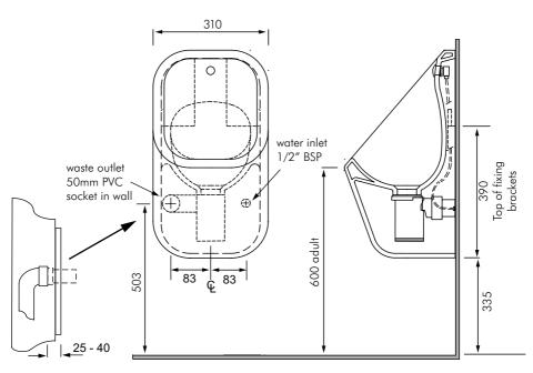
Recess 50mm socket into wall
