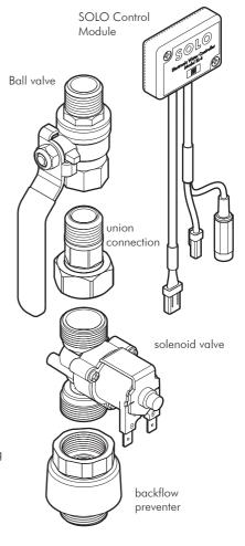
The backflow preventer provides the necessary separation to comply with Building Act Acceptable Solutions AS1/G1, ensure there is a minimum distance of 300mm between the backflow preventer and the FFL or drain (whichever is the higher). It is fitted with a 21/min flow regulator to minimise flow.
