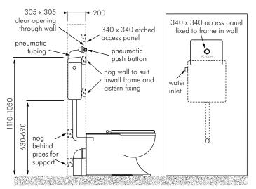
of the pan. Dimensions shown on drawing are to suit a standard WC height.
