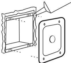
run small bead of silicon around wall to seal behind piezo plate
