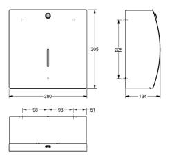
Paper towel dispenser for wall mounting, stainless steel, surface satin finished, front with InoxPlus surface refinement for the reduction of finger marks and better cleaning characteristics (easy to clean), material thickness 1.5 mm, curved front cover, cylinder lock with Franke standard key, inspection window on front, loading capacity 300 - 400 pcs. of paper depending on convolution, includes stainless steel screws and dowels.
