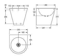
The Centinel washbasin is manufactured from 1.25 mm thick grade EN 1.4301 (304) stainless steel polished to a satin finish. The bowl is prepared with no tap hole and supplied with a 32 mm flush grated waste only (no overflow can be fitted). Complete with joggle strip and bottom access panel for fixing (using screws) and plumbing connections.
