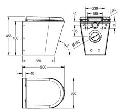
Floor standing WC pan with shroud to the floor, stainless steel, surface satin finished, material thickness 1.6 mm, flushing certificated to EN 997, concealed flushing rim with min. 4 litre flushing capacity, with a shrouded 100 mm diameter horizontal 'P' trap outlet, pressed seat area tapered towards centre, all edges curved, fixing with included mounting plate conform to EN 33, includes safety screws. 4 litre flush EN997 approved.
