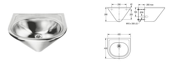
Single wash basin for wall mounting, stainless steel, surface satin finished, material thickness 1.2 mm, with 3 threaded rods for mounting through the wall via a service room, seamless welded bowl, 40 mm tap ledge, without taphole, without overflow, 1 1/4" flat perforated waste, includes hidden mounted siphon DN 32.
