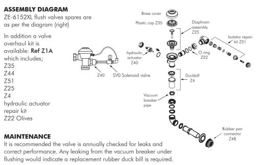
It is recommended the valve is annually checked for leaks and correct performance. Any leaking from the vacuum breaker under flushing would indicate a replacement rubber duck bill is required.
