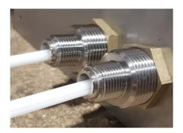
STEP 5:Once the rods are cut to the correct length the plate can be fitted. Take care to align the rods as they slide into the cavity of the push button.
