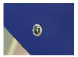
STEP 1: There are four M4 rivnuts inserted into the blue frame near the top edge.
